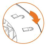
Adjust the camera modules' position and angle and place the dome cover on the camera. Secure the dome cover to the camera base using the screws included with the camera. See the camera's QSG for more information. Complete the installation by reattaching the magnetic cover over the camera dome.
