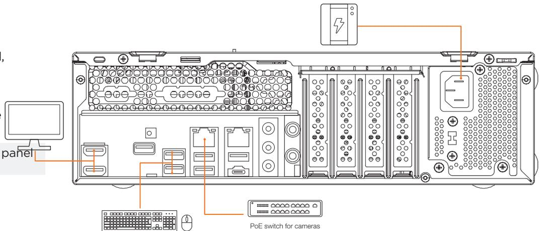
2. Connect the server to an appropriate power source. A UPS system (600VA or higher) is recommended.
