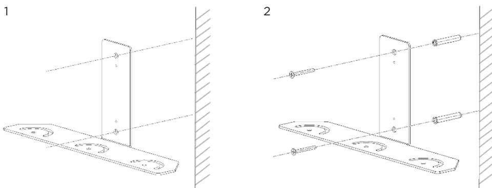
Use the bracket as a template to mark and drill the necessary holes in the wall. \*NOTE: wall anchors are for illustration only, and are not included.
