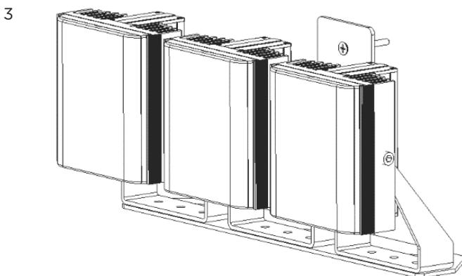
With the bracket secured to the wall attach the illuminators with the supplied M6 nuts and bolts. For each illuminator attach the center bolt first then rotate the illuminators to the required horizontal position, then secure with the remaining nut and bolt in one of the outer holes.
